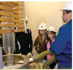
Career Day at our Joffre, Alberta, site included a laboratory demonstration of the entire polyethylene film-making process. Students watched as the film was blown out of the extruder die, cooled and finally wound onto a cardboard core.
